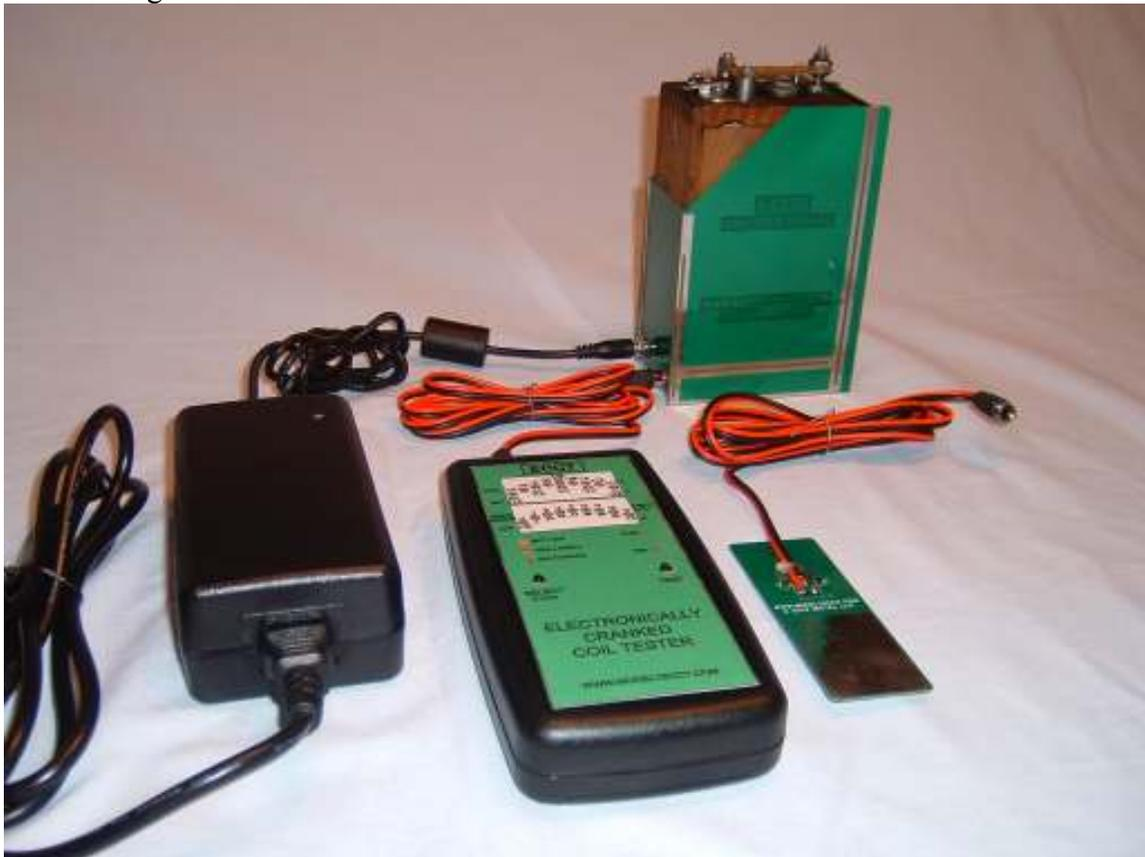
Figure 4 – ECCT, Coil Probe, Coil Test Fixture and Power Supply
