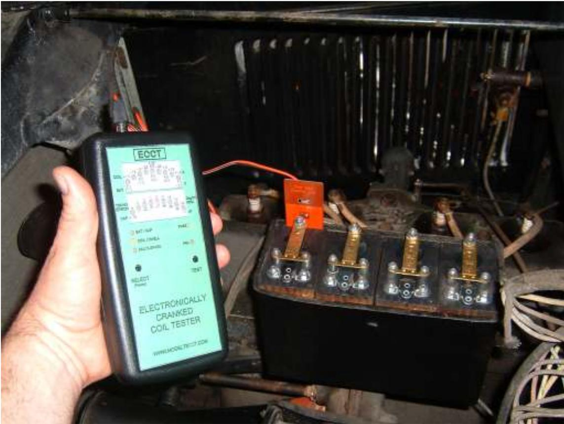
Figure 3 – The Electrically Cranked Coil Tester (ECCT) Prototype
